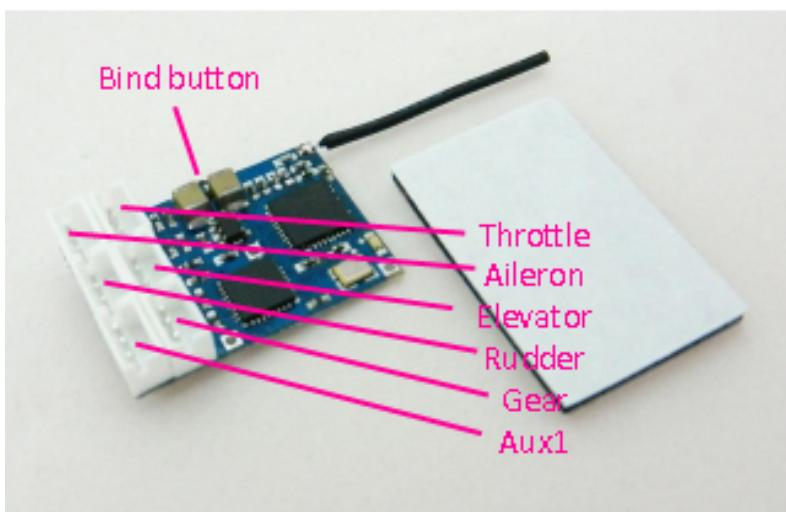
**The 6 channel Micro Light – with JST-SH 1.0mm pitch connectors.**
