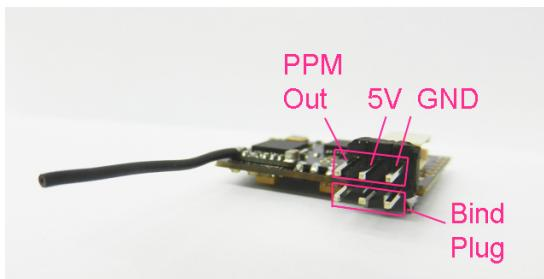
This receiver does not allow for connection of servos or a speed control. It is designed to provide a PPM stream suitable for use by a flight controller.
