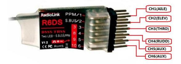
PWM signal working mode, 6channel
